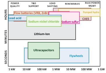
Common storage technologies and broad application categories plotted by typical system capacity and discharge time, as reported in the DOE Global Energy Storage Database [DOE, 2016].
