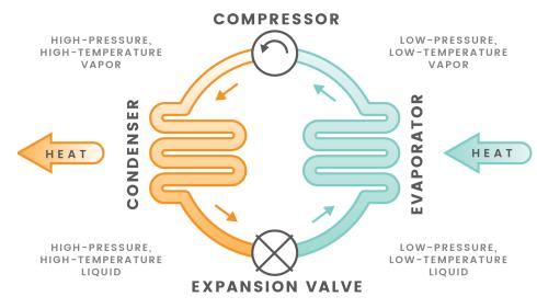
Figure 2: The refrigeration cycle in heating mode. Adapted from [3].
