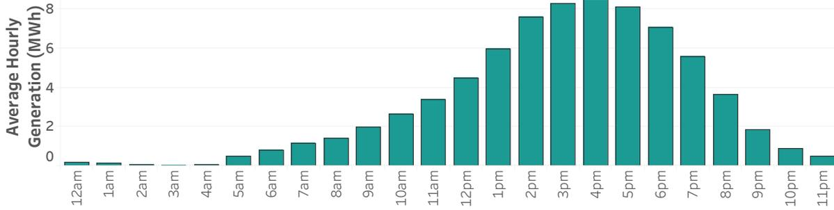
**Figure 2: Average hourly generation from the Sun Peak Generating Station.** The plant typically meets peak afternoon loads. It ran an average of 5.4 hours each time it started up between 2016 and 2018 and had a capacity factor of 1.3 percent. Batteries or solar+storage can serve a similar role on the grid.
