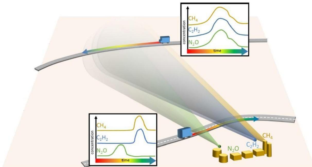
**Figure A.1.** Illustration of the tracer-tracer release technique using mobile measurement. The spatiotemporal offset of  $\text{N}_2\text{O}$  vs.  $\text{C}_2\text{H}_2$  and methane ( $\text{CH}_4$ ) in the near transect, compared to offsets at the far downwind transect, can indicate the relative location of the methane release — namely directly near the  $\text{C}_2\text{H}_2$  release point. Source: Adapted<sup>2</sup> from Roscioli et al. (2015).
