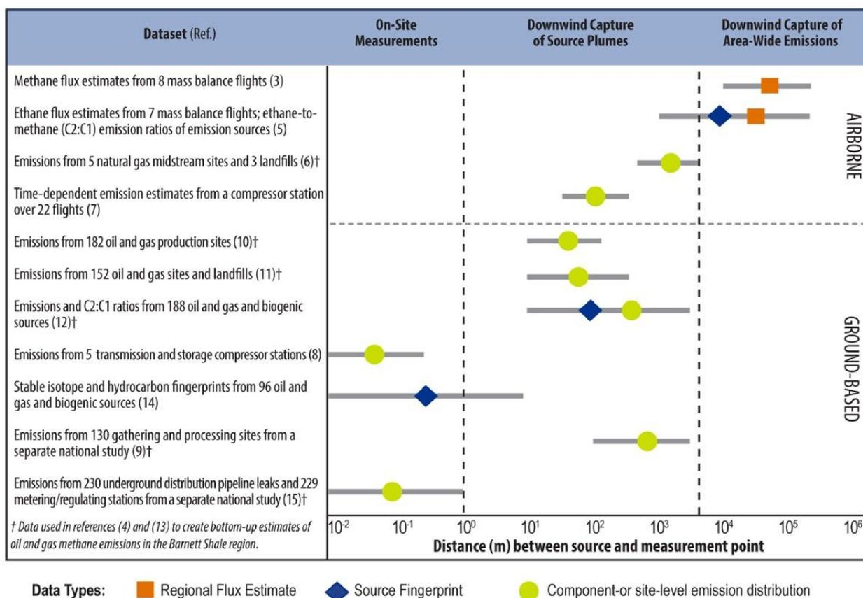
**Figure 3.2** Spatial scales of measurements taken over the course of the Barnett Shale Coordinated Campaign. Source: Reprinted with permission<sup>3</sup> from Harriss et al. (2015).
