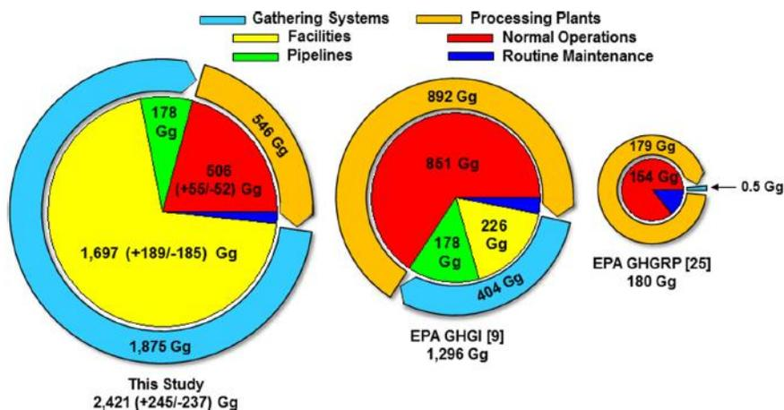
**Figure 3.6.** Gathering system and processing plant methane emissions derived from Marchese et al. (2015) with comparisons to the U.S. EPA GHGI and GHGRP. Source: Reproduced with permission<sup>12</sup> from Marchese et al. (2015).
