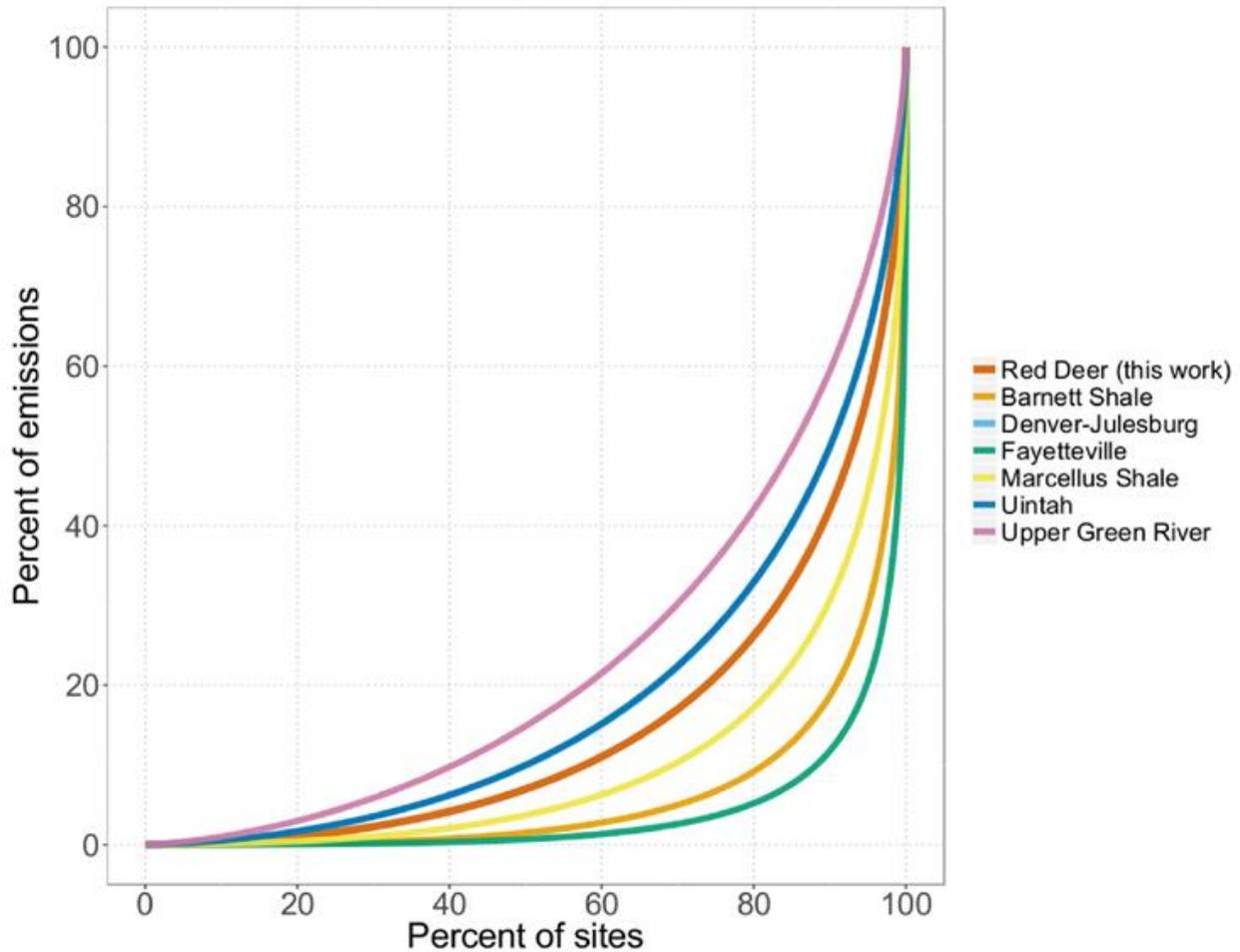
**Figure 3.3.** Lorenz curve of the distribution of emissions from emitting sites in various oil and gas producing regions in the United States and Canada where ground-based measurements have been reported. Source: Reproduced<sup>4</sup> from Zavala-Araiza et al. (2018).
