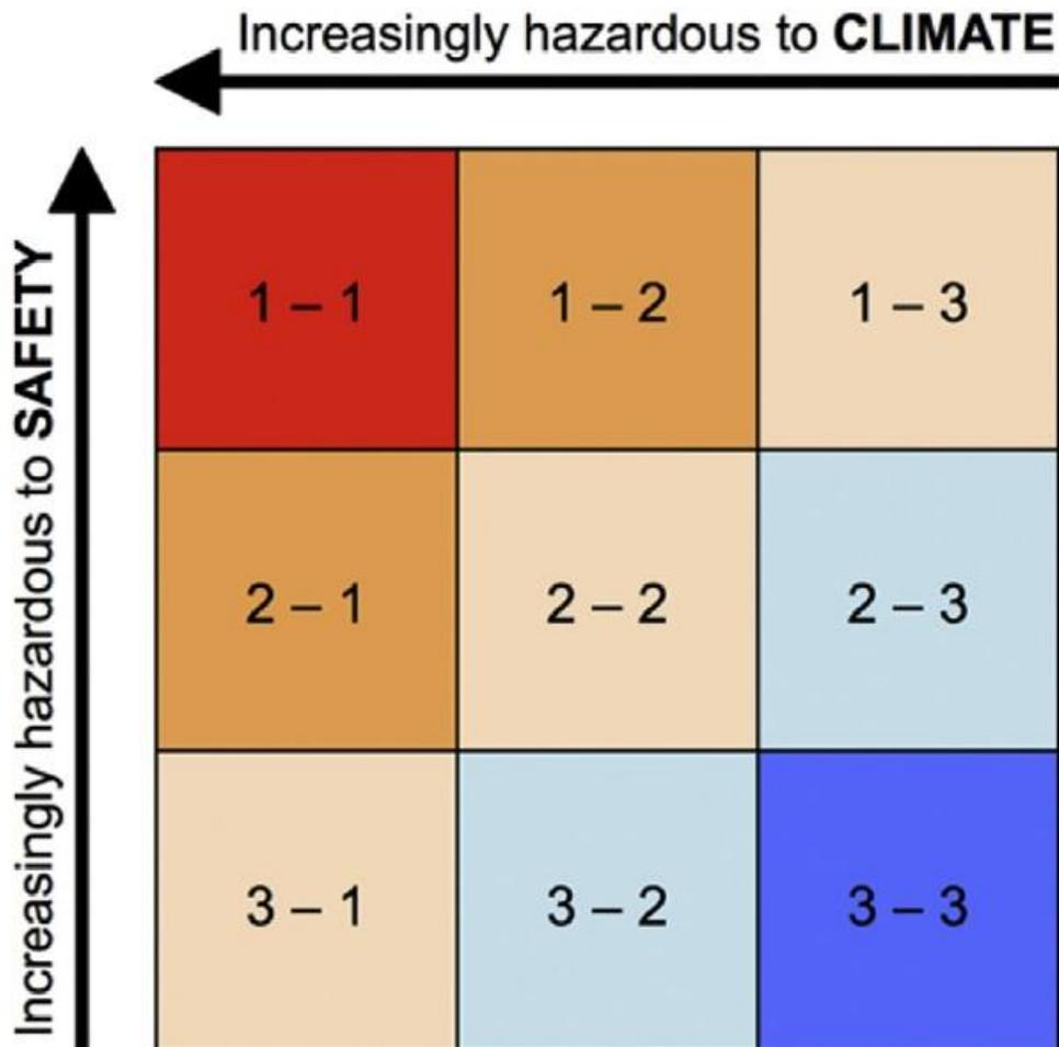
**Figure 3.9.** Framework to balance risk of natural gas leaks on climate and for local safety concerns. Deeper red colors represent leaks that are both a higher safety hazard and are large leaks. Deeper blue colors indicate overall lower risk to both safety and climate. Source: Reproduced with permission<sup>18</sup> from Hendrick et al. (2016).
