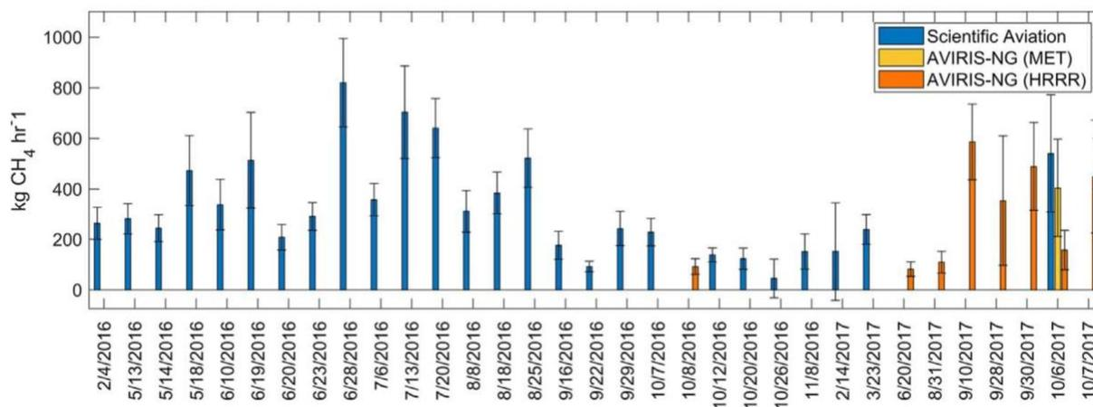
**Figure 3.8.** Time-series of methane emissions estimates from the McDonald Island UGS facility. Source: Reproduced<sup>15</sup> from Thorpe et al. (2020).
