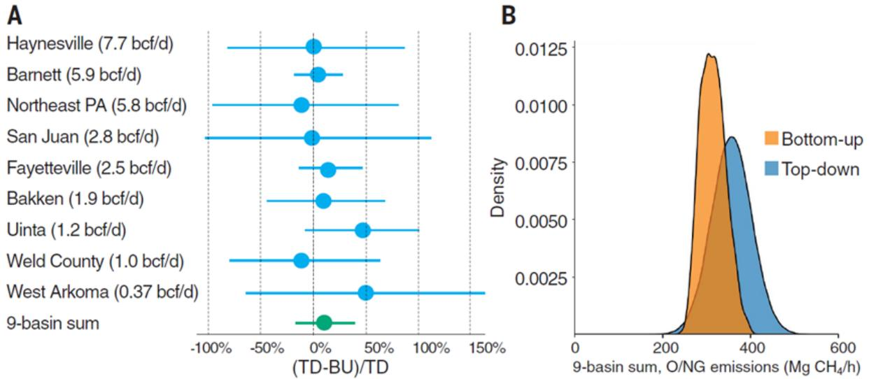
**Figure 3.1.** Comparison of top-down (TD) and bottom-up (BU) site-level estimates for nine major oil and gas producing basins when emission probability distributions were integrated into bottom-up site-level estimates. (A) Top-down normalized difference between TD and BU site-level emissions by region. Error bars represent 95% CI. (B) Probability densities for nine basin sum of TD and BU site-level estimates. Source: Reproduced from Alvarez et al. (2018) with permission<sup>2</sup>.
