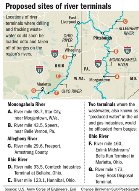
Figure 1. Proposed sites of river terminals for loading and unloading produced water by barge in the Allegheny, Monongahela, and Ohio Rivers. Figure source: Hohey, 2021.
