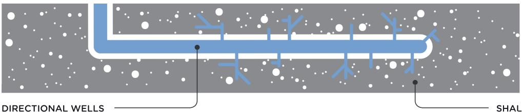
refer to wells that are deviated from the original vertical wellbore at a high angle to target a specific location. For instance, shale gas wells are drilled vertically and then laterally into the shale formation to produce oil or natural gas.
